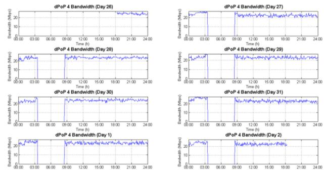
Fig. 4. TCP bandwidth results for dPoP #4.
