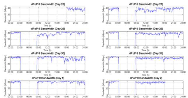
Fig. 5. TCP bandwidth results for dPoP #8
