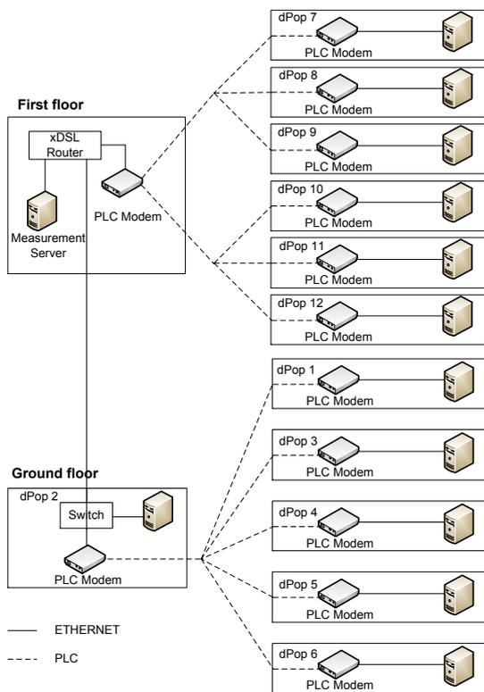
Fig. 3. “Centre de la Vila” network topology. Floors are connected through Ethernet to extend the HomePlug AV coverage beyond passive elements, such as circuit breakers and residual-current devices.
